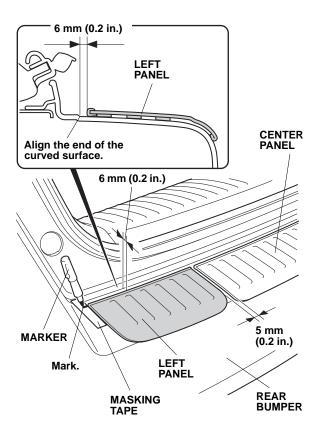
Peel back all of the adhesive backings, and tape them to the front of the left panel using pieces of masking tape.
