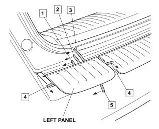
13. Using the rubber roller, apply firm pressure to the left panel, especially at the ends, as shown.
