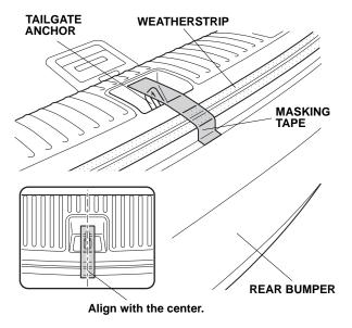
3. Position the center panel on the rear bumper, and align it with the center mark on the masking tape as shown.
