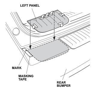
12. While pressing the left panel firmly with the palm of your hand, slowly and carefully remove the adhesive backings in the order shown.
