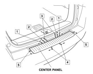
8. Remove the masking tape. Using the rubber roller, apply firm pressure to the center panel, especially at the ends, as shown.
