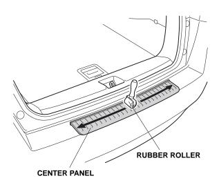
Position the left panel on the rear bumper and align it with the center panel. Attach a piece of masking tape to the rear bumper at the edge of the left panel. Using a marker, mark the masking tape at the measurement shown. Remove the left panel.
